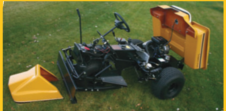
Front cover easily removes while seat and rear housing tilt back for easy service and maintenance
